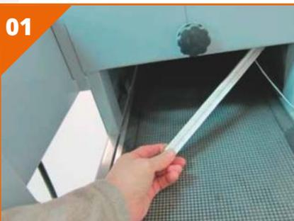
01 Remove the lamp, including reflector, from the process machine.
