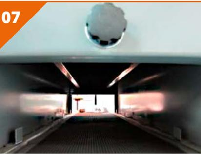
The reflector and assembly can now be re-fitted to the machine.
