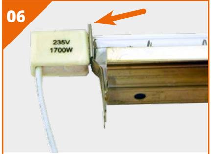
Press the top of the "spade" down until the elbow/bend sits on the same feature at the base of the reflector end clips
