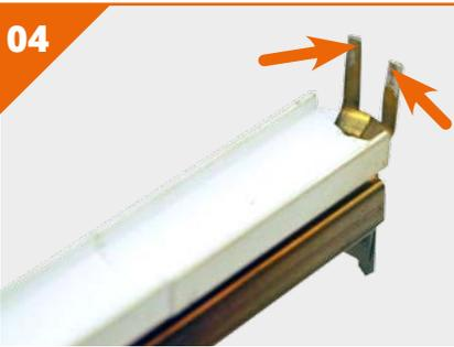
Use the pliers to straighten the end clips and the file or emery paper the cut ends to remove any burrs.
