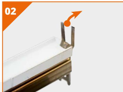
02 Completely cut the upper section of the fixed metal clip at both ends using the metal cutters.
